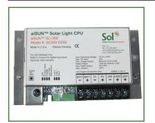
aiSUN<sup>™</sup> is the Central Processing Unit of a solar light. Featuring advanced microprocessor control and a highly efficient design, aiSUN<sup>™</sup> controls and monitors solar lights with more flexibility and capability than ever before. aiSUN<sup>™</sup> is an LED driver with an integrated solar charge controller.
